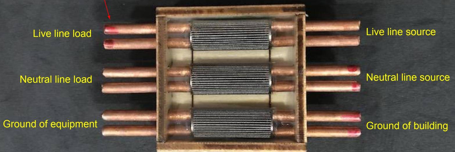
Pinch both copper rods of each polarity together and solder your lead to both simultaneously. As this is 20mm<sup>2</sup>, a large iron is necessary. (We use 150 Watts.)
